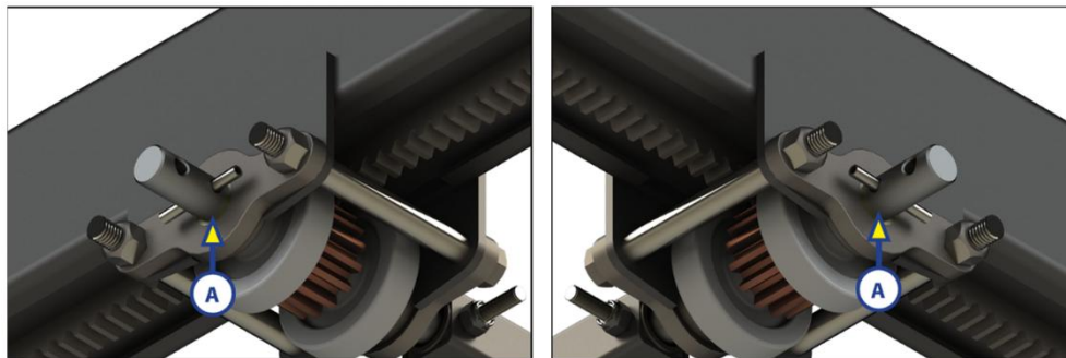
Figure 26. Gear Pack lubrication points - exterior.
