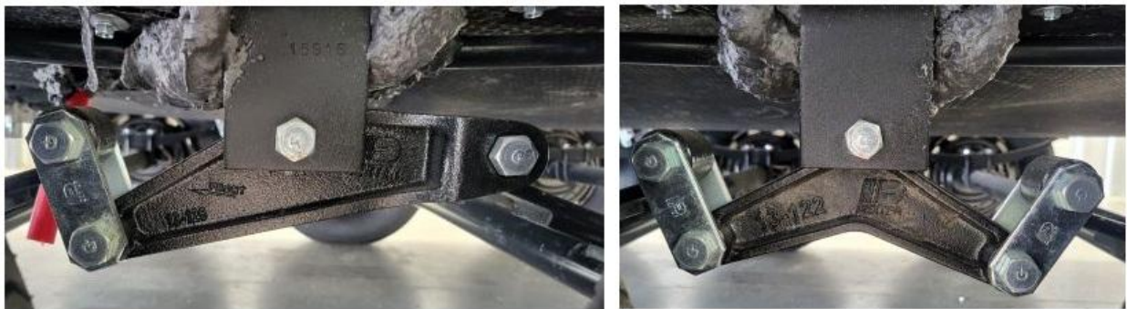
Figure 5. Dual equalizer arrangement. The forward end of the trailer is to the left. The middle axle does not have a shackle to connect the leaf spring to the forward equalizer.
