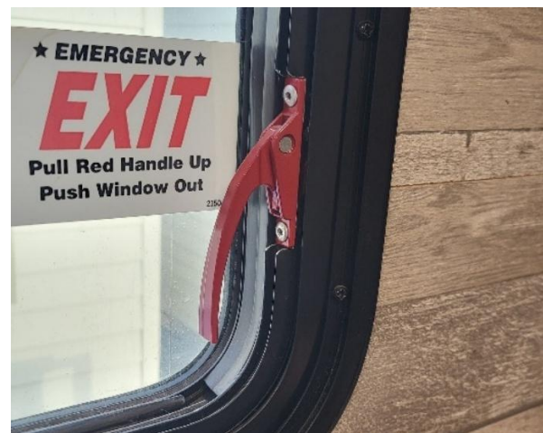
Figure 12. Pull-Lever style latch on an emergency exit. Pull the lever out, away from base, to disengage latch. Push window out.
