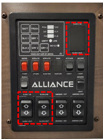
Figure 22. Monitor panel with slide-out controls (and potential slide-out controls) highlighted.
