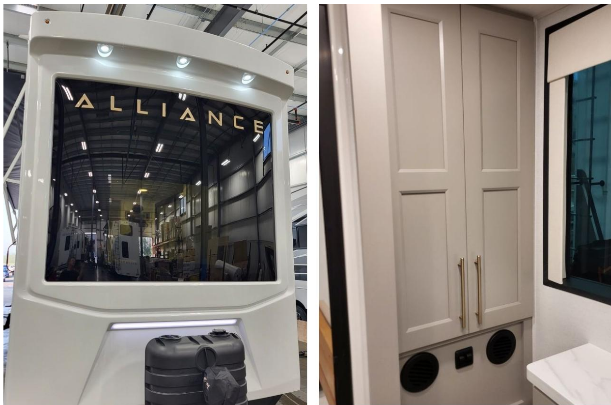
Figure 56. The exterior front porch and docking lights (left) as well as the switch location inside the front bathroom (right, below doors.)
