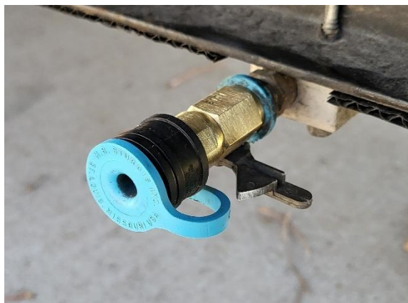
Figure 18. External propane quick connect, with flow lever in the "off" position.
