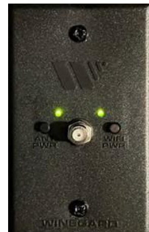
Figure 54. Winegard booster switch, with booster and Wifi enabled.
