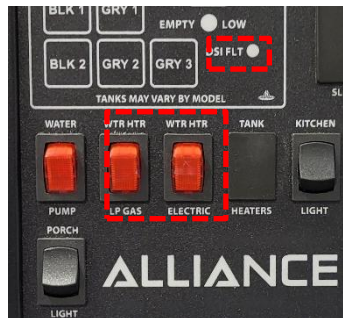
Figure 66. The water heater power switches on the main Monitor Panel. The DSI FLT light is highlighted on the upper right. These are also shown in Figure 39C and D.
