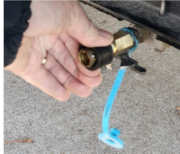
Figure 19. Pushing the retaining ring to accept an appliance connector.
