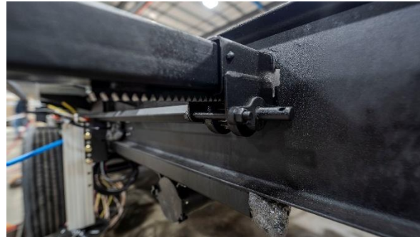
Figure 24. Through-frame gear pack.
