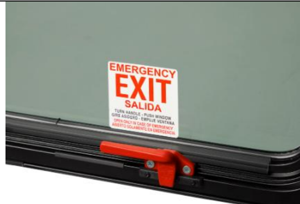
Figure 11. Rotation-Lever style latch on an emergency exit. Rotate the handle up into the window area to disengage the latch. Push window out.
