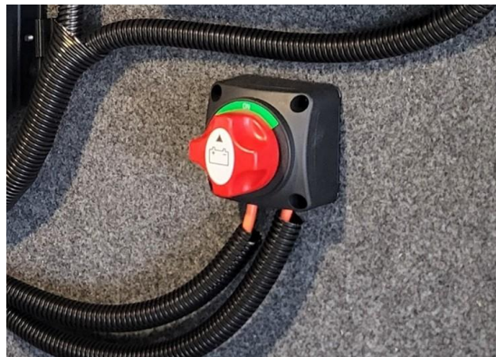
Figure 35. Battery disconnect switch as mounted on a different trailer model.
