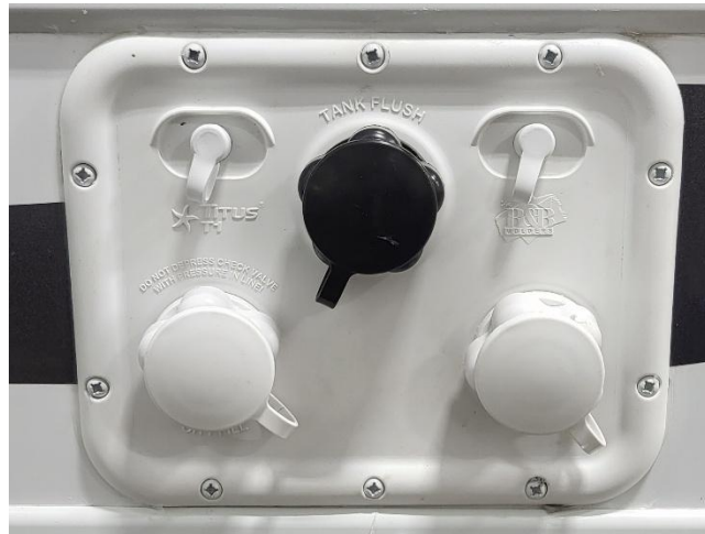
Figure 57. Titus T1 Water Management System panel. It is located on the Off Door Side (ODS) of the trailer near the rear.
