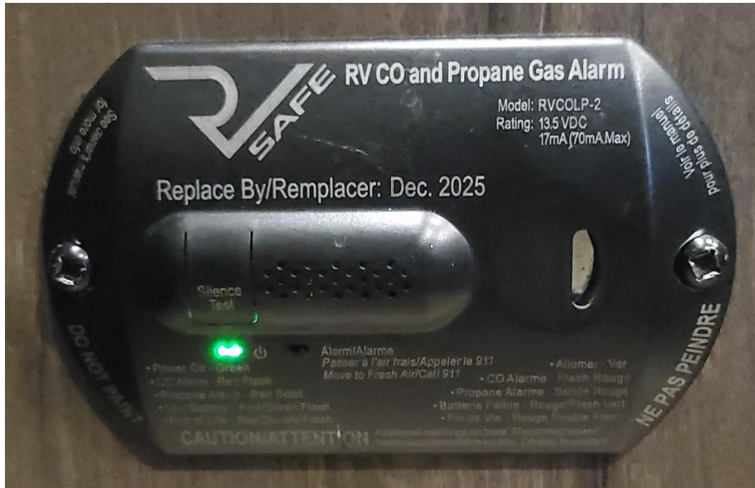
Figure 15. Wall mounted Carbon Monoxide (CO) and Propane alarm. These will be mounted near floor level, usually near stairs.
